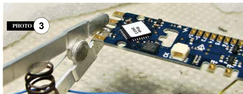
Photo 3: Clamp the other end of the SMD resistor to the decoder terminal and solder it in place. A heat sink clamp or an alligator clip from a test lead can be used to hold the resistor in place. It is best to solder this to the control terminal and not the V+ power source.
